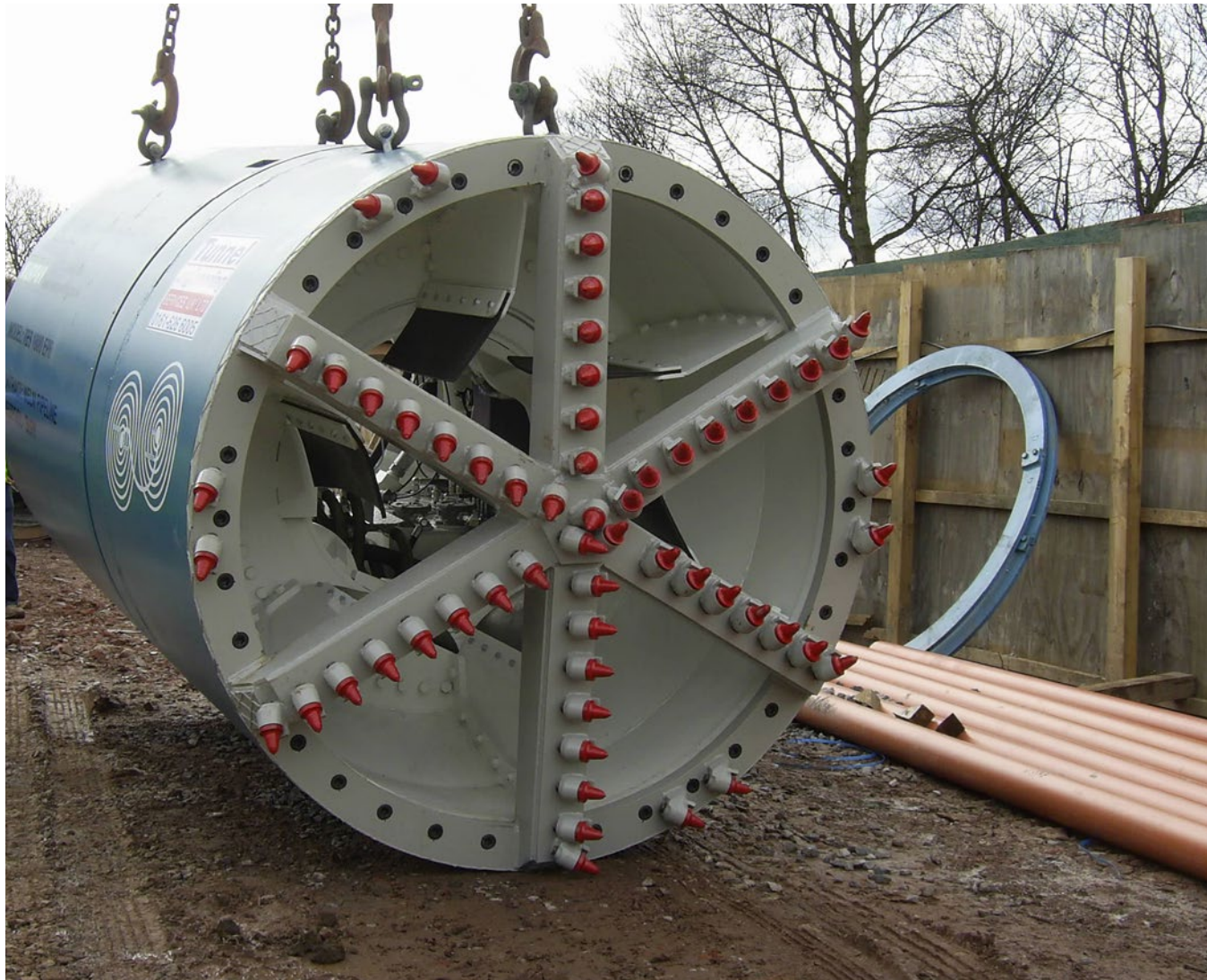
Typical example of a small tunnel boring machine of the size being proposed for the Project.
