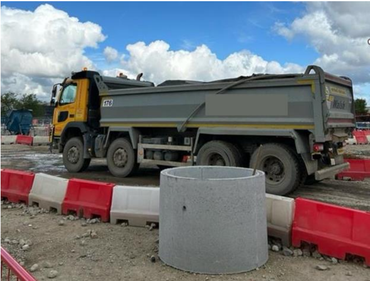
Plate 2-11 Image of a typical construction vehicle for the movement of bulk materials
