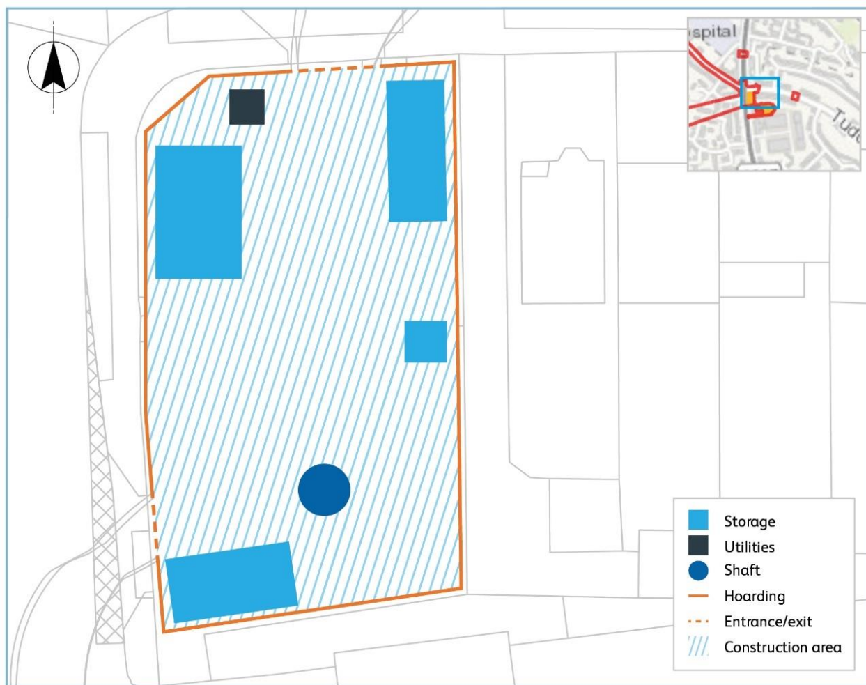
Plate 2.7 An indicative illustration of the Tudor Drive site temporary compound layout
