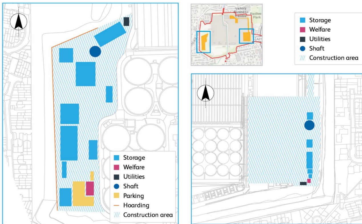
Plate 2.4 An indicative illustration of the Mogden STW temporary site compound layout at the Western and Eastern Work Area
