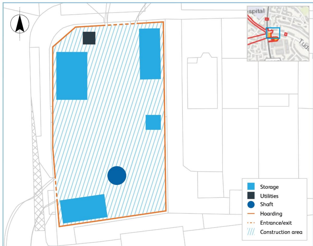
Plate 2.6 An indicative illustration of the Tudor Drive temporary site compound layout
