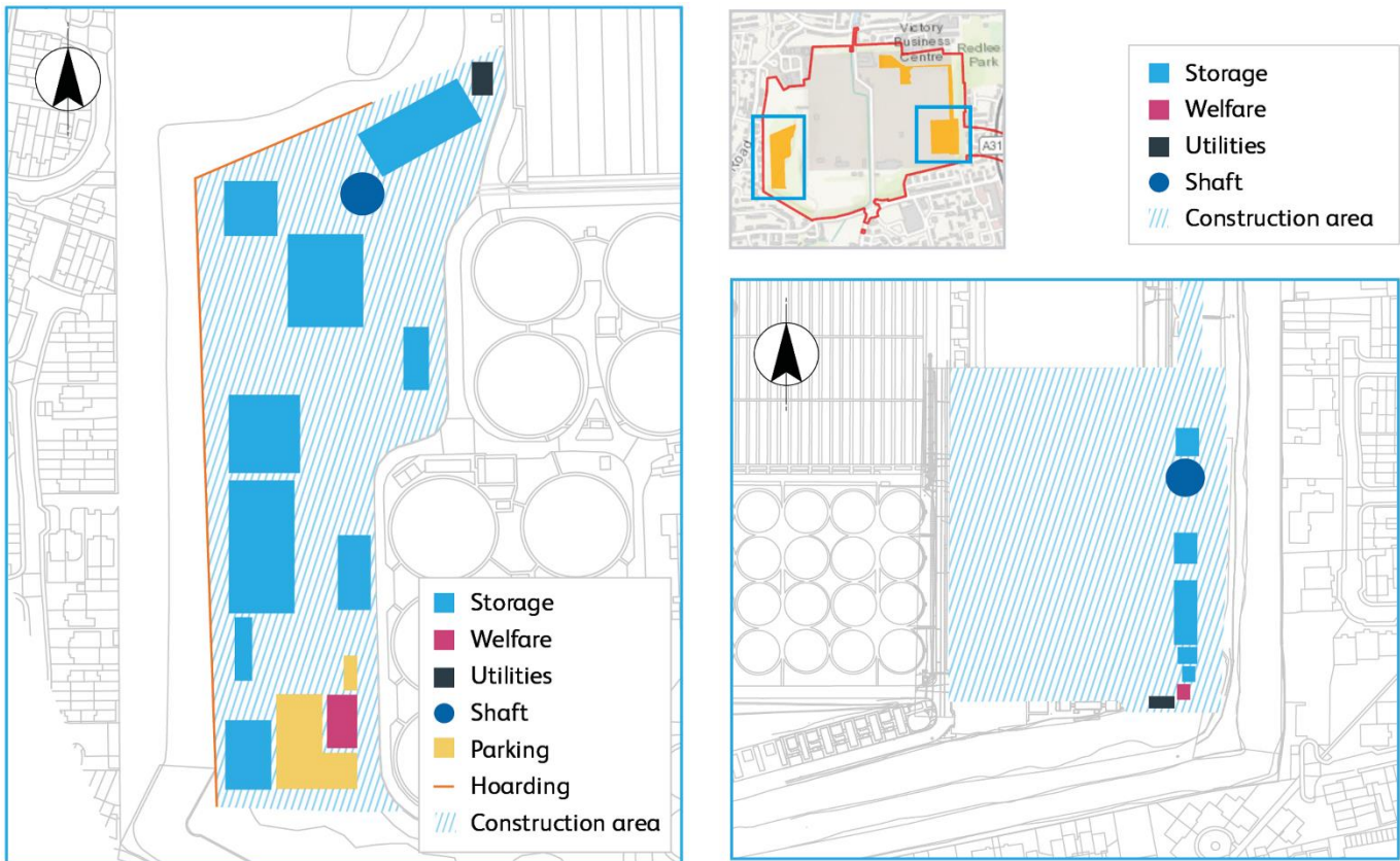
Plate 2.3 An indicative illustration of the Mogden STW temporary site compound layout at the Western and Eastern Work Area
