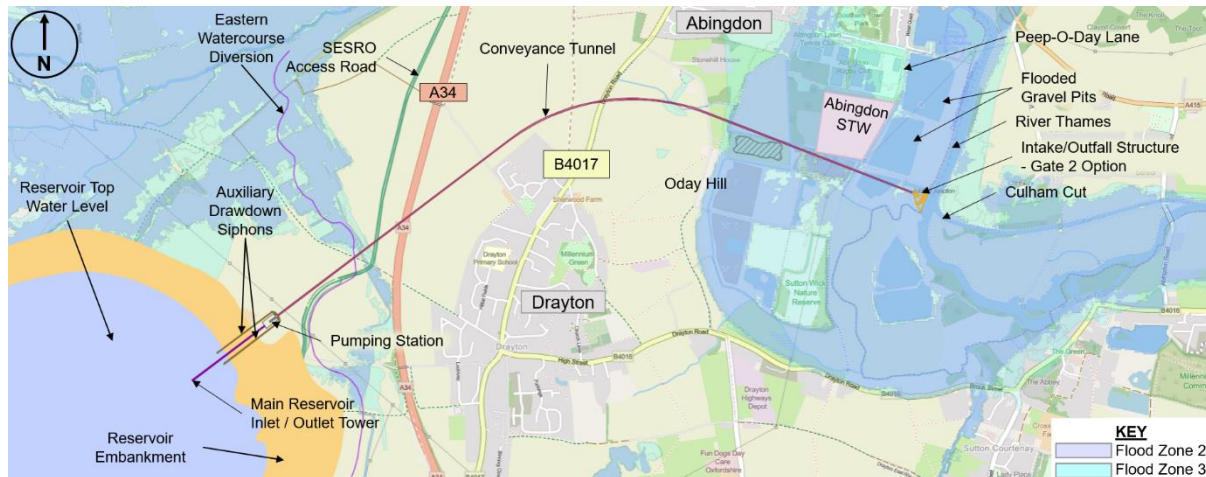
Figure 8.6: Emergency Discharge Option C – Tunnel Only
