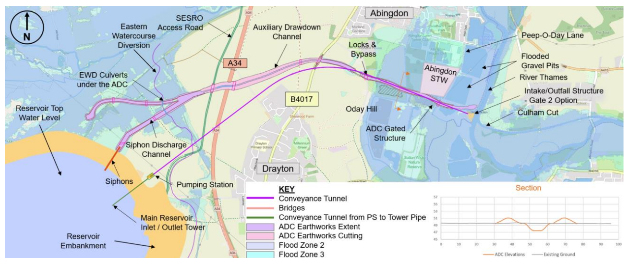
Figure 8.1: Emergency Discharge Option A – ADC and Tunnel
